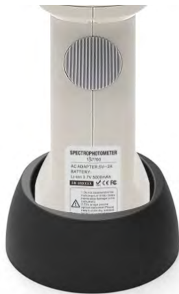
4. Place the base safely to ensure that the whiteboard is not dirty
